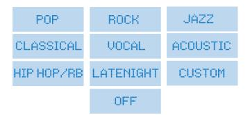
2. You can also access the EQ setting through the Menu as discussed in the Menu Setting of AiOS. The Custom setting allows for a curve of 15 bands of the following frequencies with a +/- 12 range per band. You can also tweak any preset to your liking and save that as your preset through the use of the Android and iOS control apps. You may find adjusting the EQ setting through the control app easier and more intuitive.
