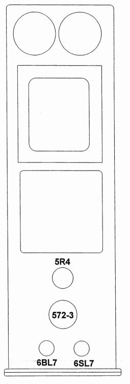
Large pins on SV-572-3 tube MUST be inserted into the large holes in the sockets! These pins are on the front of the amplifier.
