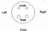
\*\*\* WARNING: When installing 572 tubes; Large pins orient towards the front of the chassis. Failure to follow these guidelines will result in severe damage to your equipment.
