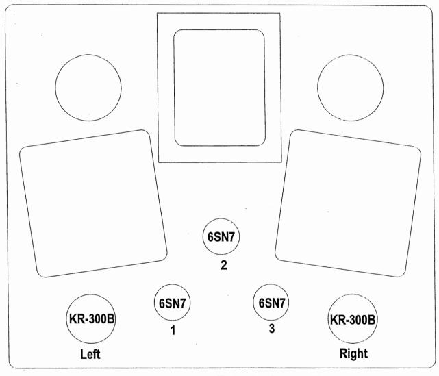
Large pins on KR-300B tube MUST be inserted into the large holes in the sockets!
