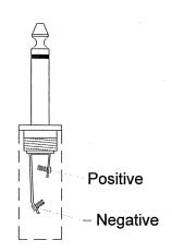
Insert meter plug into bias jack. monitor for ~90mA (+-10mA) reading on VOM or DC current meter.
