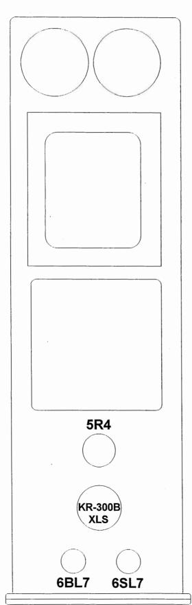
Large pins on KR-300B tube MUST be inserted into the large holes in the sockets! These pins are on the right side of the amplifier.
