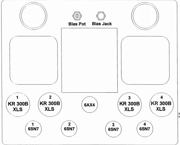
Large pins on KR-300B tube MUST be inserted into the large holes in the sockets! These pins are on the right side of the amplifier.
