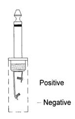
Insert meter plug into bias jack. Meter should read 65-75 mA. Wall voltage and other variables can affect bias reading.
