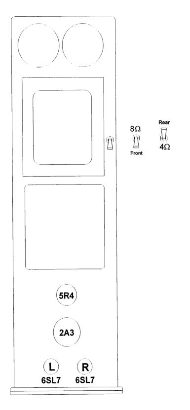
\*\*\* WARNING: When installing 2A3 tubes; Large pins orient towards the front of the chassis. Failure to follow these guidelines will result in severe damage to your equipment.
